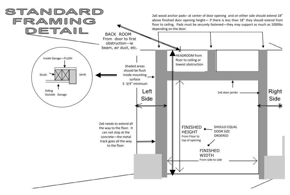
FRAMING SHOULD BE SQUARE; FLOOR LEVEL/HEADER LEVEL; MINIMUM OF 2in AT BOTTOM (6in AT TOP) OF DOOR ON EITHER SIDE NEEDED—IF STEM WALL IS CLOSER CEMENT WILL NEED TO BE CHIPPED AWAY
